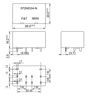
PC board mounting hole layout (BOTTOM VIEW)
