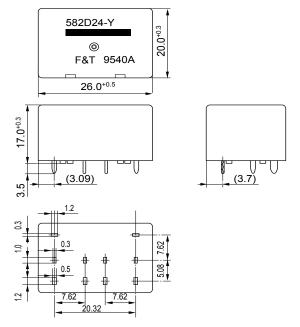
PC board mounting hole layout (BOTTOM VIEW)
